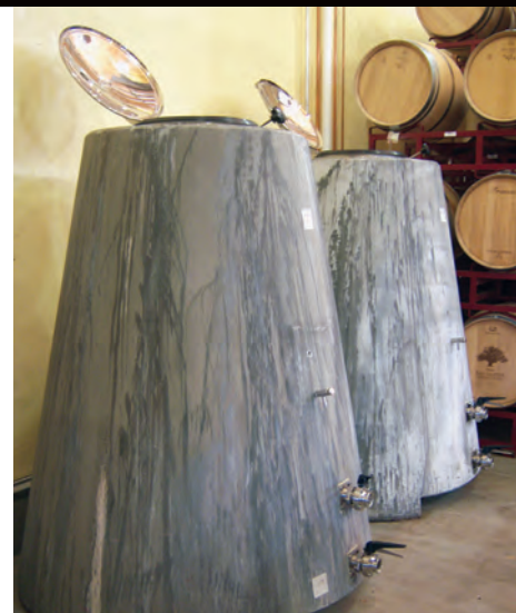
Two of the four Vino Vessel concrete fermentation tanks at the winery.
