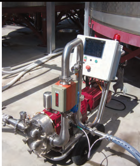
The RapidFil Cellar-Mate semi-automated wine transfer system.
